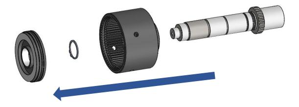
13. Piston and clutch shaft should be assembled in clutch case with snap ring after o-ring is replaced and well greased.
