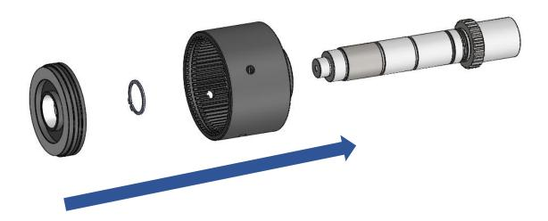
14. Spring, washer and snap ring should be assembled in a row.
