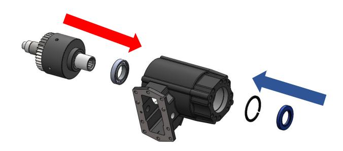
20. O-ring on the PTO cover should be greased before bearing is placed inside on the cover. Next, PTO cover should be assembled on the PTO body with 4 bolts.
