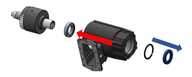
6. Snap ring and washer should be removed from the clutch shaft.
